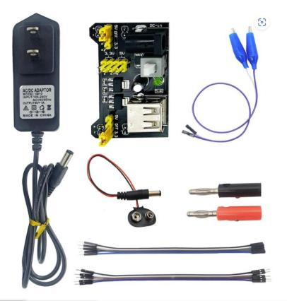
9 v AC-DC power suppy 3.3v or 5v reg pin selectable Power via USB Power by 9 v battery Different voltages or zero via rails On/off switch Built test leads with banana For < 700 ma use
